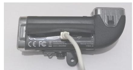
At this point, the power LED on the camera control board will turn on, indicating the battery is charging. The battery level during charging is shown through the power LED in the following way:
