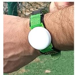
Your wrist remote allows you to trigger the recordings remotely. To do that, you simply press the top of the remote until you hear a click and a blue LED flashes for ~1 second. There are two things you need to do to use the remote:
