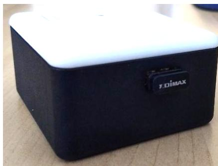
You can connect the hub to the internet using a compatible USB WiFi dongle. Insert the dongle in the USB port on the side of the hub and connect to your access point (e.g. your smartphone as a hotspot or your home router) from the “Internet access” section of the “System settings” tab of the user interface.
